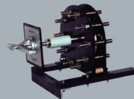
Delta-Wye Switch Assembly: 500 AMP, 2 position, 3 phase (1 deck), 25kV, 150 kV BIL, wall mount, shown with padlockable T- handle and index plate
