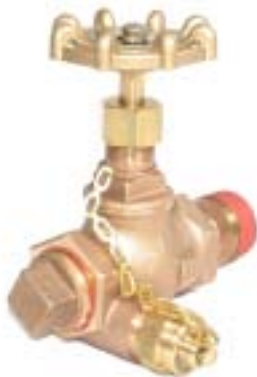
Drain Valve with Nipple & Plug Installed utilizing Loctite Vibra-Seal 516 Sealant on all joints
