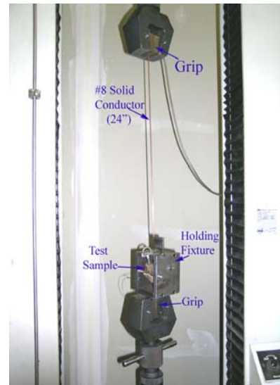
Pullout Test (Keeper)
