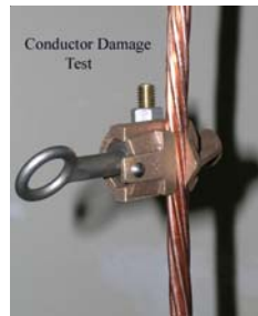
Conductor Damage Test
