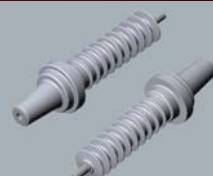
1200 Series 15.2 kV, 95 kV BIL, 600 Amp "Shedded" Apparatus Bushing Removable Stud, 14.5" Creep
