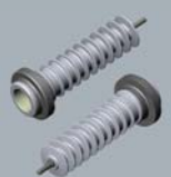
1200 Series 15.2 kV, 125 kV BIL, 200 Amp "Shedded" Bushing Well Removable Stud, 14.5" Creep
